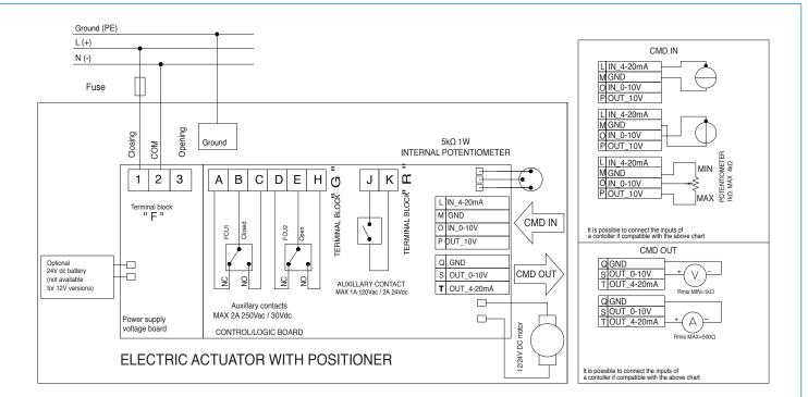
The power supply COM signal ( pin "2" terminal block "F") cannot share the same electrical command ground signal ( pin "GND" terminal block "CDM IN") or feedback ground signal (pin "GND" terminal block "CDM OUT").
